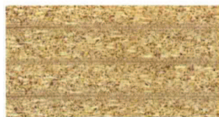
Particle board or chipboard
