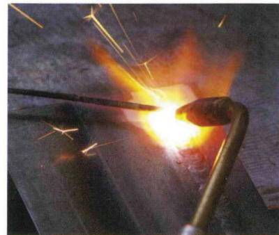
Gas welding using oxyacetylene
