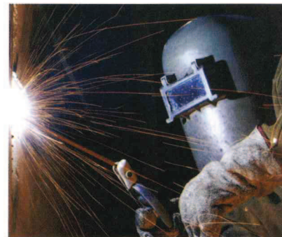
Shielded metal arc welding
