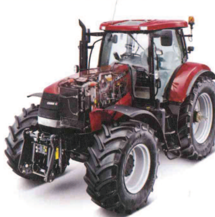
The Case-IH Puma CVX tractor is equipped with continuously variable transmission.
