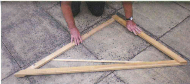
A large setsquare for setting out
