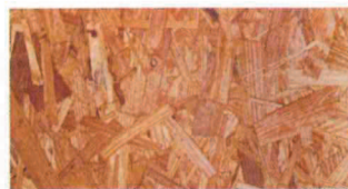
Orientated strand board (OSB)
