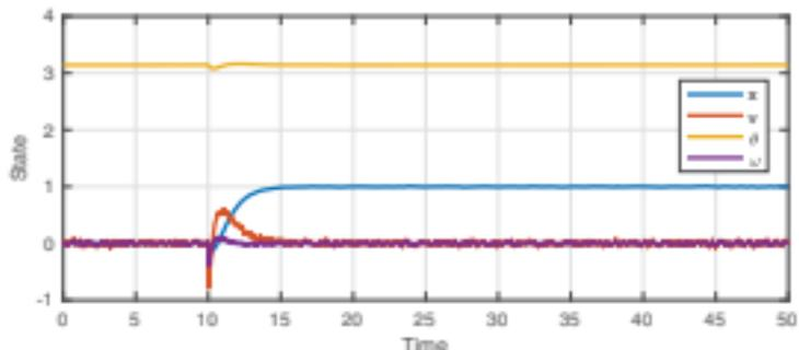
Figure 8.18 Output response using LQG feedback control.
