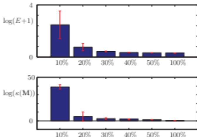
**Figure 12.4** Logarithm of the least-square error,  $\log(E+1)$  (unity is added to avoid negative numbers), and the log of the condition number,  $\log(\kappa(\mathbf{M}))$ , as a function of percentage of random measurements. For 10% measurements, the error and condition number are largest as expected. However, the variance of the results, depicted by the red bars, is also quite large, suggesting that the performance for a small number of sensors is highly sensitive to their placement.
