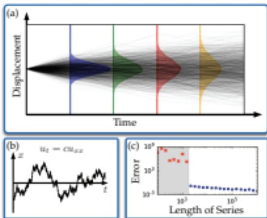
**Figure 7.8** Inferring the diffusion equation from a single Brownian motion (reproduced from Rudy *et al.* [460]). (a) Time series is broken into many short random walks that are used to construct histograms of the displacement. (b) The Brownian motion trajectory, following the diffusion equation. (c) Parameter error ( $\|\hat{\xi}^* - \xi\|_1$ ) vs. length of known time series. Blue symbols correspond to correct identification of the structure of the diffusion model,  $u_t = cu_{xx}$ .
