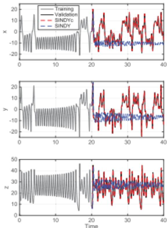
**Figure 10.3** SINDY and SINDYc predictions for the controlled Lorenz system in (10.22). Training data consists of the Lorenz system with state feedback. For the training period the input is  $w(t) = 26 - x(t) + d(t)$  with a Gaussian disturbance  $d$ . Afterward the input  $w$  switches to a periodic signal  $w(t) = 50 \sin(10t)$ . Reproduced with permission from [100].
