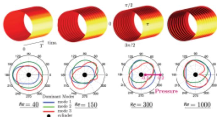
**Figure 12.19** Time dynamics of the pressure field (top panels) for flow around a cylinder for Reynolds number  $Re = 40, 150, 300$  and  $1000$ . Collecting snapshots of the dynamics reveals low-dimensional structures dominate the dynamics. The dominant three POD pressure modes for each Reynolds number regime are shown in polar coordinates. The pressure scale is in magenta (bottom left). (reproduced from Katz; et al. [319])
