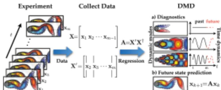
Figure 7.3 Overview of DMD illustrated on the fluid flow past a circular cylinder at Reynolds number 100. Reproduced from [317].
