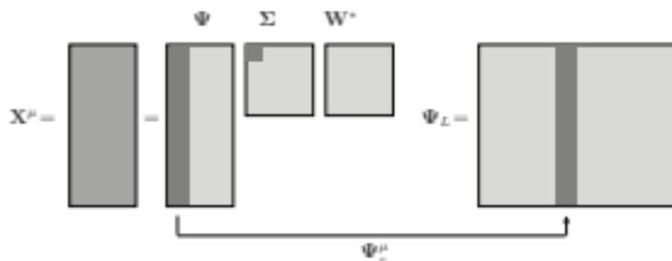
**Figure 12.17** Library construction from numerical simulations of the governing equations (11.1). Simulations are performed of the parametrized system for different values of a bifurcation parameter  $\mu$ . For each regime, low-dimensional POD modes  $\Psi_r$  are computed via an SVD decomposition. The various rank- $r$  truncated subspaces are stored in the library of modes matrix  $\Psi_L$ . This is the learning stage of the algorithm. (reproduced from Katz *et al.* [319])
