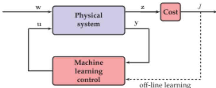
**Figure 10.5** Schematic of machine learning control wrapped around a complex system using noisy sensor-based feedback. The control objective is to minimize a well-defined cost function  $J$  within the space of possible control laws. An off-line learning loop provides experiential data to train the controller. Genetic programming provides a particularly flexible algorithm to search out effective control laws. The vector  $z$  contains all of the information that may factor into the cost.
