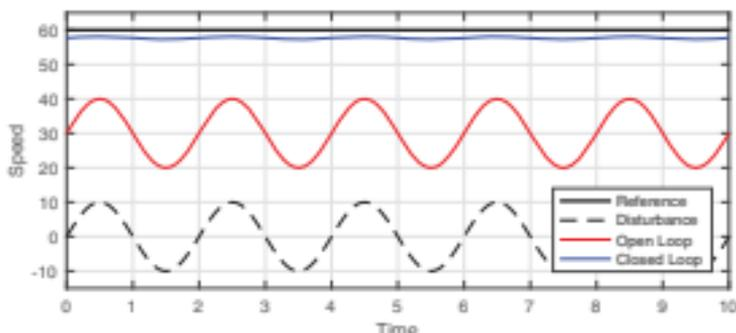
Figure 8.5 Open-loop vs. closed-loop cruise control.
