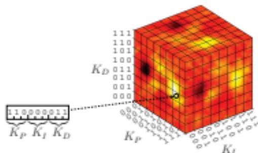
**Figure 10.6** Depiction of parameter cube for PID control. The genetic algorithm represents a given parameter value as a *genetic sequence* that concatenates the various parameters. In this example, the parameters are expressed in binary representation that is scaled so that **000** is the minimum bound and **111** is the upper bound. Color indicates the cost associated with each parameter value.
