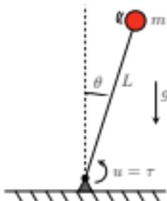
**Figure 8.8** Schematic of inverted pendulum system.
