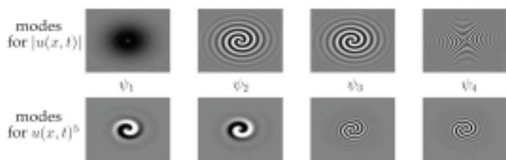
**Figure 11.13** First four POD modes associated with the rotating spiral wave  $|u(x, y)|$  (top row) and  $u(x, t)^5$  (bottom row). Unlike our previous example, the first four modes do not capture all the variance to numerical precision, thus requiring more modes for accurate approximation. The domain considered is  $x \in [-20, 20]$  and  $y \in [-20, 20]$ .
