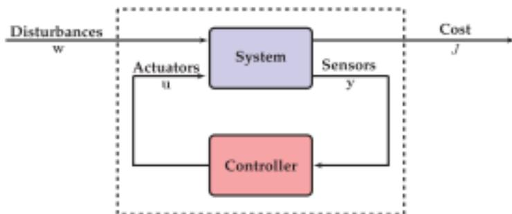
**Figure 8.2** Standard framework for feedback control. Measurements of the system,  $y(t)$ , are fed back into a controller, which then decides on the appropriate actuation signal  $u(t)$  to control the system. The control law is designed to modify the system dynamics and provide good performance, quantified by the cost  $J$ , despite exogenous disturbances and noise in  $w$ . The exogenous input  $w$  may also include a reference trajectory  $w_r$  that should be tracked.
