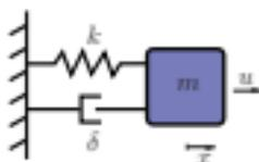
Figure 8.22 Spring-mass-damper system.
