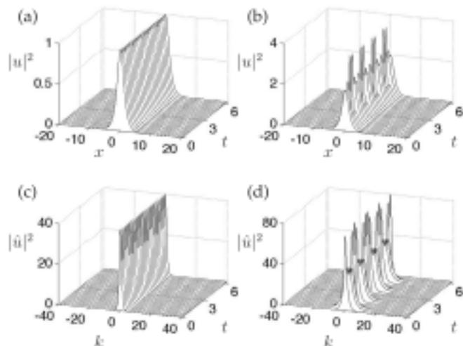
**Figure 11.4** Evolution of the (a)  $N = 1$  and (b)  $N = 2$  solitons. Here steady-state ( $N = 1$ , left panels (a) and (c)) and periodic ( $N = 2$ , right panels (b) and (d)) dynamics are observed and approximately 50 and 200 Fourier modes, respectively, are required to model the behaviors.
