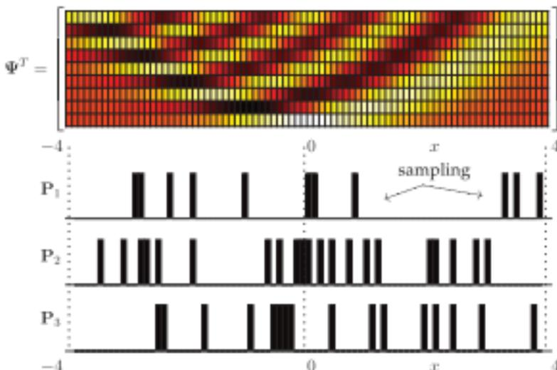
**Figure 12.1** The top panel shows the first 10 modes of the quantum harmonic oscillator considered in (11.25) and (11.26). Three randomly generated measurement matrices,  $\mathbf{P}_j$  with  $j = 1, 2$  and  $3$ , are depicted. There is a 20% chance of performing a measurement at a given spatial location  $x_j$  in the interval  $x \in [-4, 4]$  with a spacing of  $\Delta x = 0.1$ .
