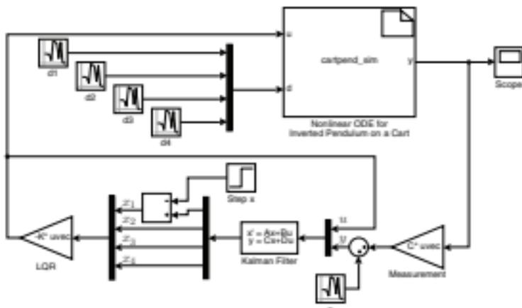
Figure 8.17 Matlab Simulink model for sensor-based LQG feedback control.
