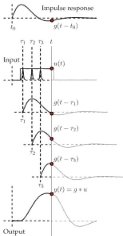
Figure 8.8 Convolution for a single-input, single-output (SISO) system.
