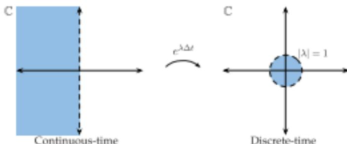
**Figure 8.7** The matrix exponential defines a conformal map on the complex plane, mapping stable eigenvalues in the left half plane into eigenvalues inside the unit circle.
