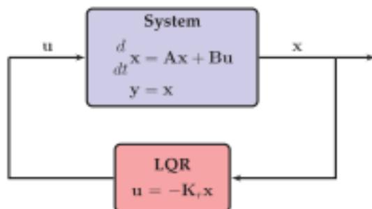
**Figure 8.9** Schematic of the linear quadratic regulator (LQR) for optimal full-state feedback. The optimal controller for a linear system given measurements of the full state,  $y = x$ , is given by proportional control  $u = -K_r x$  where  $K_r$  is a constant gain matrix obtained by solving an algebraic Riccati equation.
