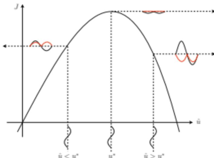
**Figure 10.17** Schematic illustrating extremum-seeking control on a static objective function  $J(u)$ . The output perturbation (red) is in phase when the input is left of the peak value (i.e.  $u < u^*$ ) and out of phase when the input is to the right of the peak (i.e.  $u > u^*$ ). Thus, integrating the product of input and output sinusoids moves  $\hat{u}$  towards  $u^*$ .
