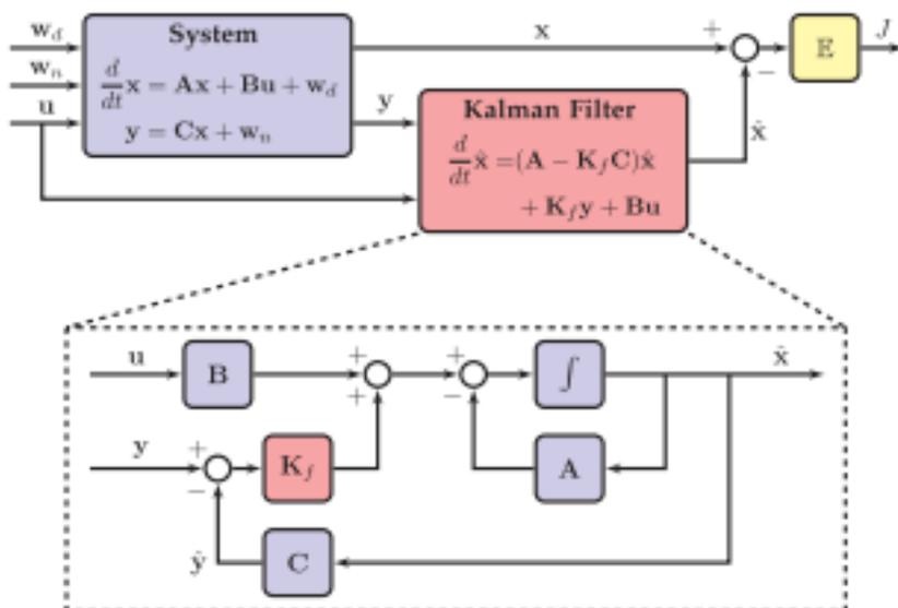
**Figure 8.10** Schematic of the Kalman filter for full-state estimation from noisy measurements  $y = Cx + w_n$  with process noise (disturbances)  $w_d$ . This diagram does not have a feedthrough term  $D$ , although it may be included.
