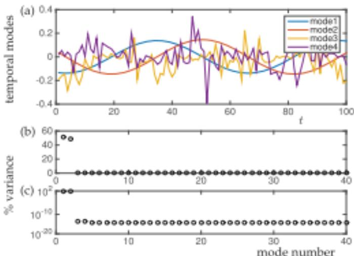
**Figure 11.10** (a) First four temporal modes of the matrix  $V$ . To numerical precision, all the variance is in the first two modes as shown by the singular value decay on a normal (b) and logarithmic (c) plot. Remarkably, the POD extracts exactly two modes (See Fig. 11.11) to represent the rotating spiral wave.
