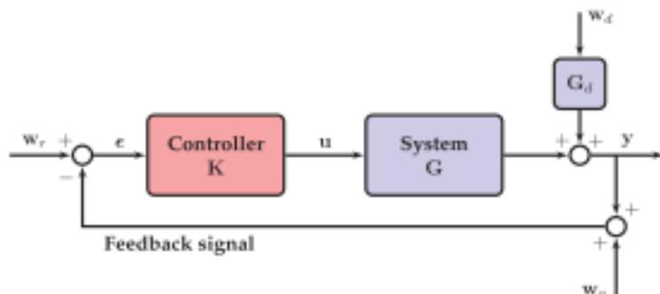
**Figure 8.26** Closed-loop feedback control diagram with reference input, noise, and disturbance. We will consider the various transfer functions from exogenous inputs to the error  $\epsilon$ , thus deriving the loop transfer function, as well as the sensitivity and complementary sensitivity functions.
