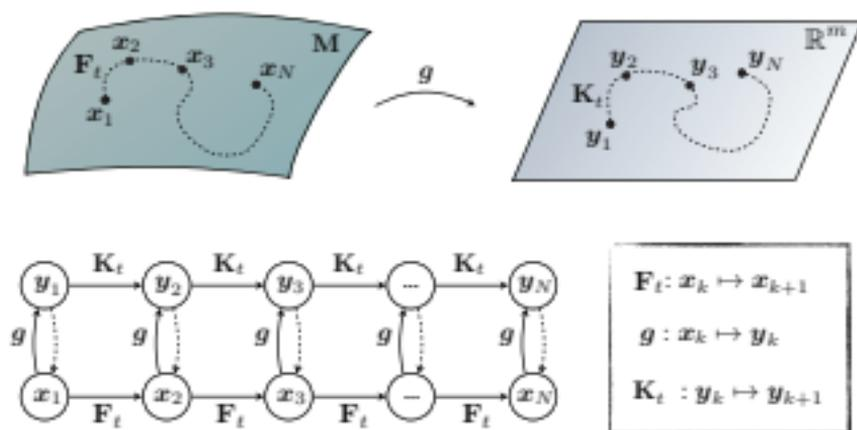
**Figure 7.10** Schematic illustrating the Koopman operator for nonlinear dynamical systems. The dashed lines from  $y_k \rightarrow x_k$  indicate that we would like to be able to recover the original state.
