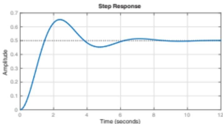
Figure 8.25 Step response of spring-mass-damper system.
