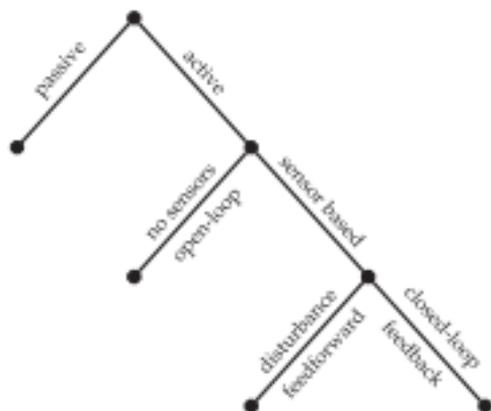
**Figure 8.1** Schematic illustrating the various types of control. Most of this chapter will focus on closed-loop feedback control.
