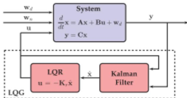
**Figure 8.11** Schematic illustrating the linear quadratic Gaussian (LQG) controller for optimal closed-loop feedback based on noisy measurements  $y$ . The optimal LQR and Kalman filter gain matrices  $K_f$  and  $K_y$  may be designed independently, based on two different algebraic Riccati equations. When combined, the resulting sensor-based feedback remains optimal.
