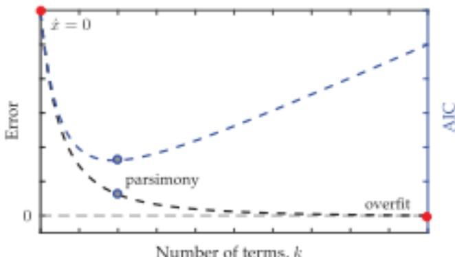
**Figure 7.9** Illustration of model selection using SINDy and information criteria, as in Mangan et al. [362]. The most parsimonious model on the Pareto front is chosen to minimize the AIC score (blue circle), preventing overfitting.
