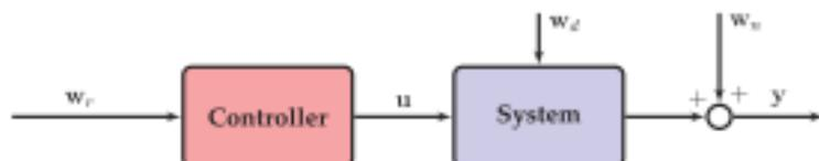
**Figure 8.3** Open-loop control diagram. Given a desired reference signal  $w_r$ , the open-loop control law constructs a control protocol  $u$  to drive the system based on a model. External disturbances ( $w_d$ ) and sensor noise ( $w_n$ ), as well as unmodeled system dynamics and uncertainty, are not accounted for and degrade performance.
