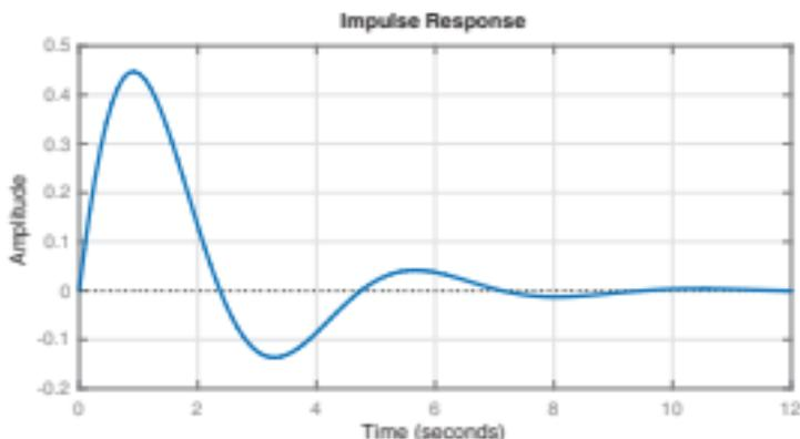
Figure 8.24 Impulse response of spring-mass-damper system.
