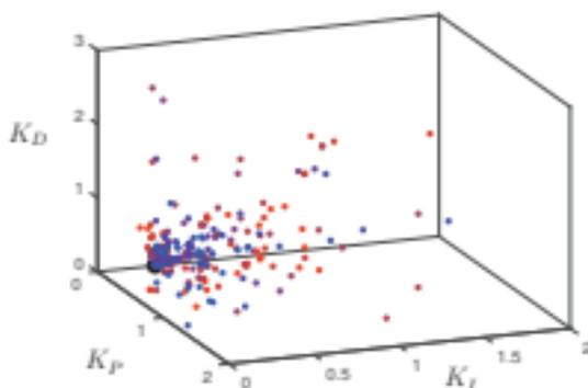
**Figure 10.12** PID gains generated from genetic algorithm. Red points correspond to early generations while blue points correspond to later generations. The black point is the best individual found by GA.
