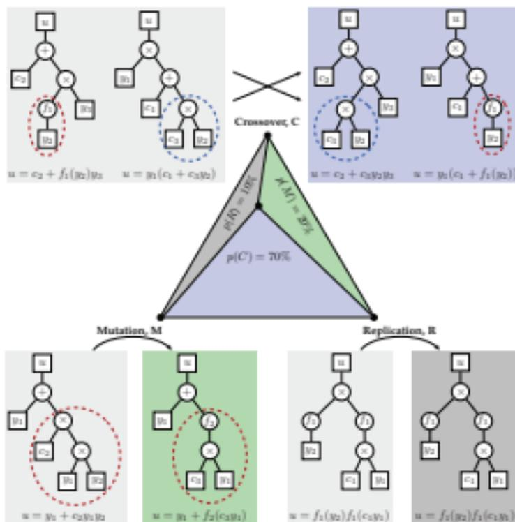
**Figure 10.9** Genetic operations used to advance function trees across generations in genetic programming control. The relative selection rates of replication, crossover, and mutation are  $p(R) = 0.1$ ,  $p(C) = 0.7$ , and  $p(M) = 0.2$ , respectively.
