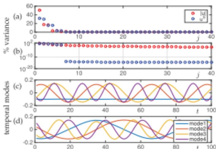
**Figure 11.12** Decay of the singular values on a normal (a) and logarithmic (b) scale showing that the function  $|u(x, t)|$  produces a slow decay while  $u(x, t)^5$  produces an  $r = 6$  approximation to numerical accuracy. The first four temporal modes of the matrix  $V$  are shown for these two functions in (c) and (d) respectively.
