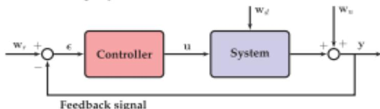
**Figure 8.4** Closed-loop feedback control diagram. The sensor signal  $y$  is fed back and subtracted from the reference signal  $w_r$ , providing information about how the system is responding to actuation and external disturbances. The controller uses the resulting error  $e$  to determine the correct actuation signal  $u$  for the desired response. Feedback is often able to stabilize unstable dynamics while effectively rejecting disturbances  $w_d$  and attenuating noise  $w_n$ .
