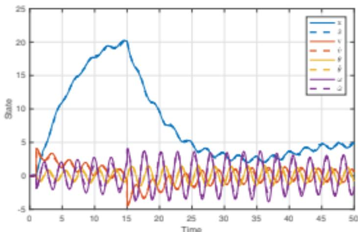
**Figure 8.16** The true and Kalman filter estimated states for the pendulum on a cart system.
