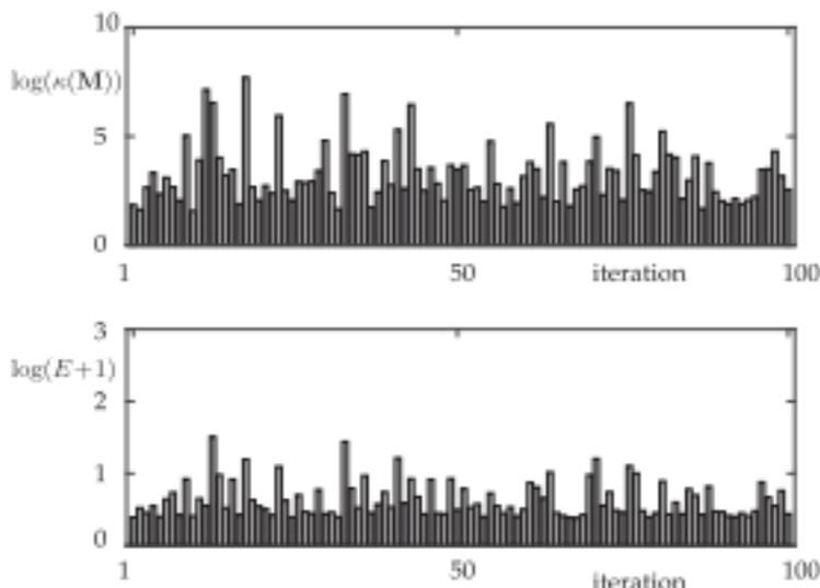
**Figure 12.13** Condition number and least-square error to test function (12.11) over 100 random trials that draw 20 sensor locations from the possible 55 extrema depicted in Fig. 12.12. The 100 trials produce a number of sensor configurations that perform close to the level of the condition number minimization algorithm of the last section. However, the computational costs in generating such trials can be significantly lower.
