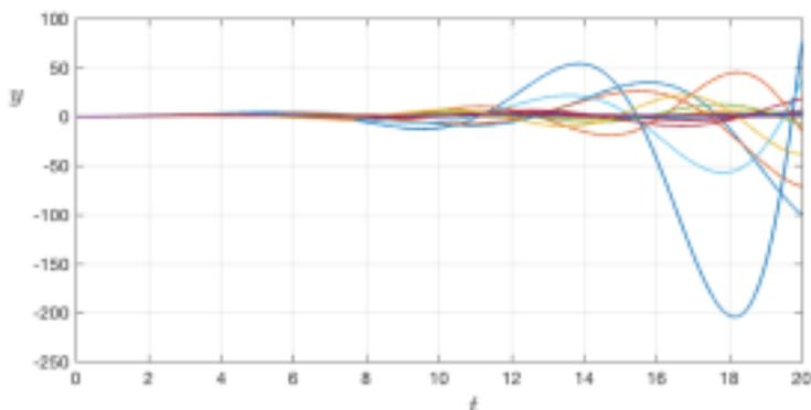
**Figure 10.13** PID controller response from first generation of genetic algorithm.
