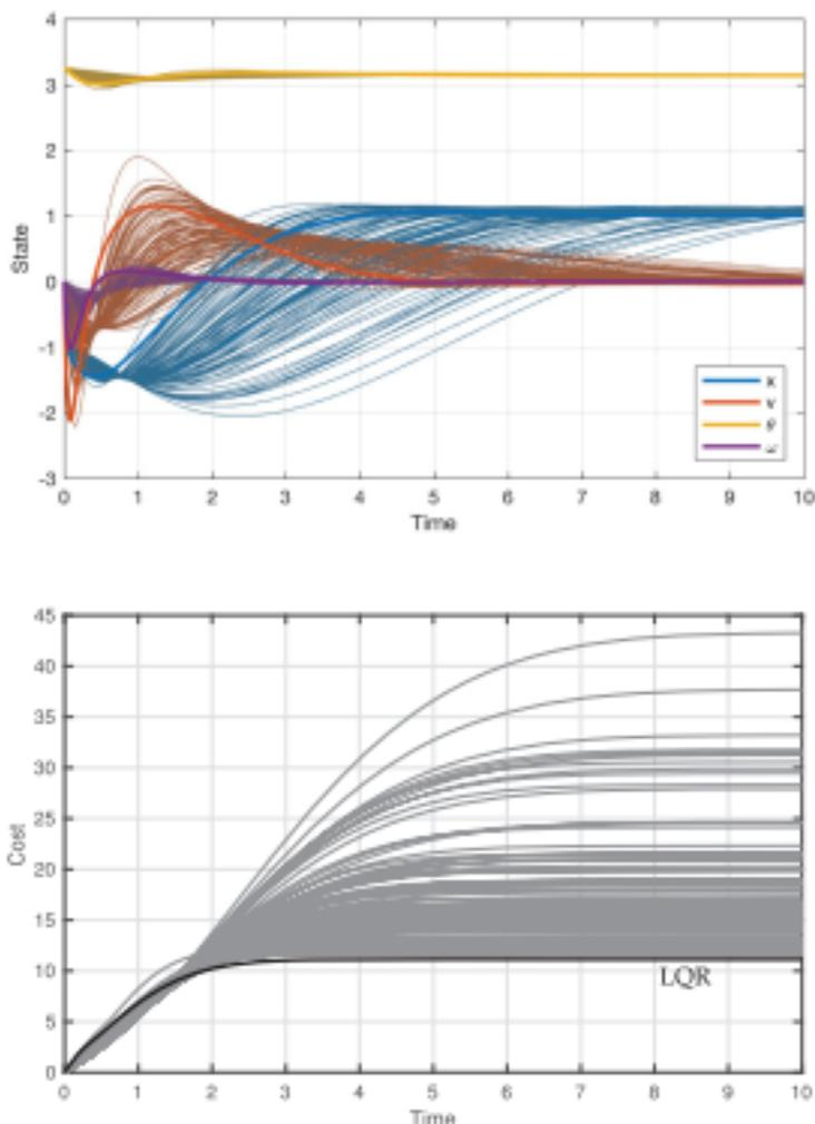
**Figure 8.14** Comparison of LQR controller response and cost function with other pole placement locations. Bold lines represent the LQR solutions.
