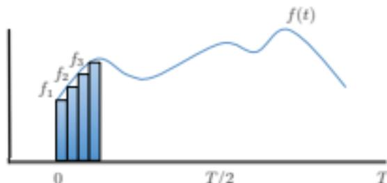
**Figure 11.6** Illustration of an implementation of the quadrature rule to evaluate the integrals  $\int_0^T f(t)dt$ . The rectangles of height  $f(t_j) = f_j$  and width  $\delta t$  are summed to approximate the integral.
