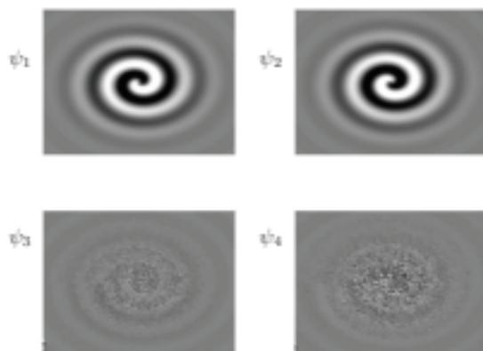
**Figure 11.11** First four POD modes associated with the rotating spiral wave  $w(x, y)$ . The first two modes capture all the variance to numerical precision while the third and fourth mode are noisy due to numerical round-off. The domain considered is  $x \in [-20, 20]$  and  $y \in [-20, 20]$ .
