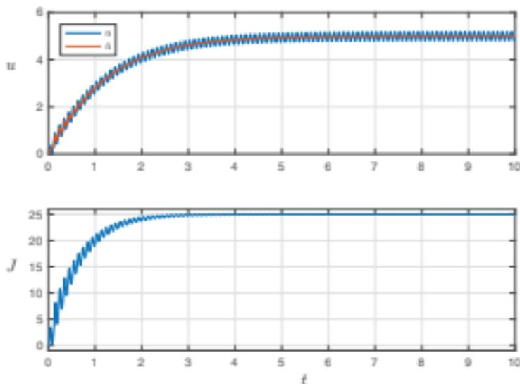
Figure 10.18 Extremum-seeking control response for cost function in (10.29).
