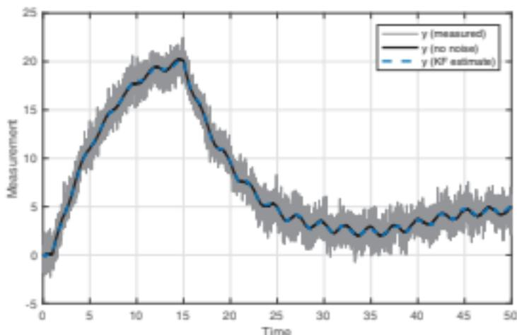
**Figure 8.15** Noisy measurement that is used for the Kalman filter, along with the underlying noiseless signal and the Kalman filter estimate.
