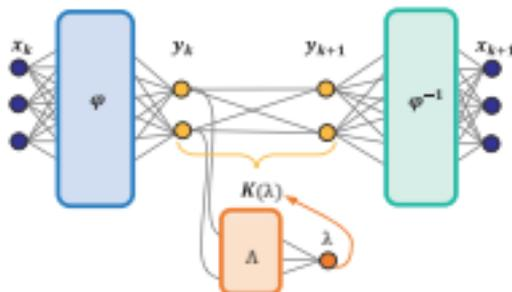
**Figure 7.14** Modified network architecture with auxiliary network to parameterize the continuous eigenvalue spectrum. A continuous eigenvalue  $\lambda$  enables aggressive dimensionality reduction in the auto-encoder, avoiding the need for higher harmonics of the fundamental frequency that are generated by the nonlinearity. Reproduced with permission from Lusch et al. [349].
