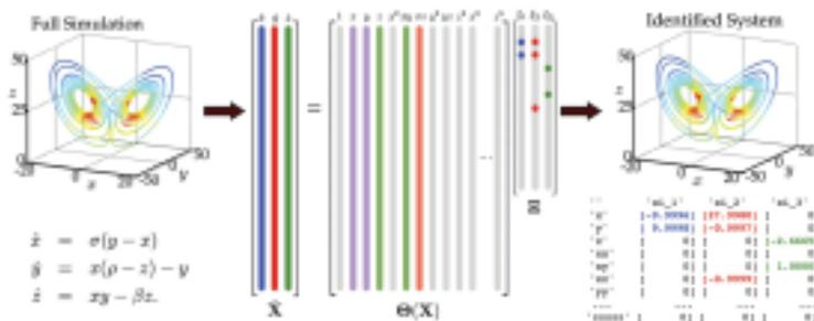
**Figure 7.4** Schematic of the sparse identification of nonlinear dynamics (SINDy) algorithm [95]. Parsimonious models are selected from a library of candidate nonlinear terms using sparse regression. This library  $\Theta(X)$  may be constructed purely from measurement data. Modified from Brunton et al. [95].
