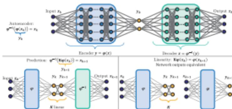
**Figure 7.13** Deep neural network architecture used to identify Koopman eigenfunctions  $\boldsymbol{\varphi}(\mathbf{x})$ . The network is based on a deep auto-encoder (a), which identifies intrinsic coordinates  $\mathbf{y} = \boldsymbol{\varphi}(\mathbf{x})$ . Additional loss functions are included to enforce linear dynamics in the auto-encoder variables (b,c). *Reproduced with permission from Lusch et al. [349].*
