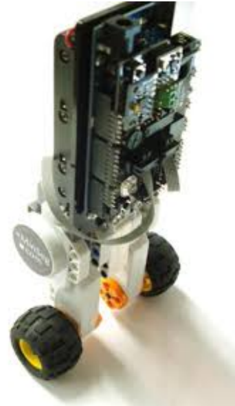
Figure 1: An example of a two-wheeled balancing robot.
